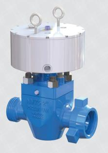
The Premium Oilfield Technologies AirForce<sup>™</sup> mud gate valve provides the user with remote bleed-off capability of standpipe lines translating to a simplified and safer user interface. Utilizing the Premium NV-7500 core design allows our valve to be one of the longest lasting valves in the industry for applications up to 7500 psi.
